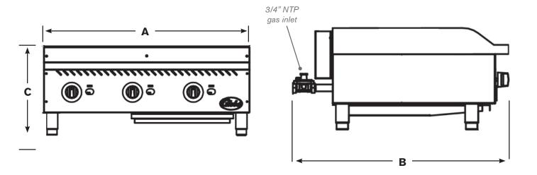
CLEARANCES These units can be installed on non-combustible countertops using the provided 3.5 inch (88.9 mm) legs or on a combustible floor using a minimum 28.5-inch (723.9 mm) tall stand. The back and both sides must be at least six inches (152.4 mm) from any combustible surface.
